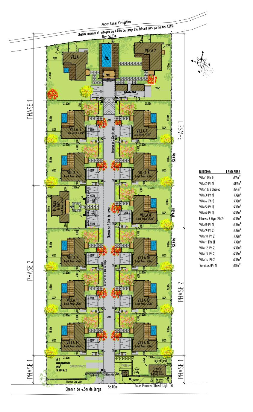
Rendered Master Site Plan - Phase 1 & 2 Scale 1:500
